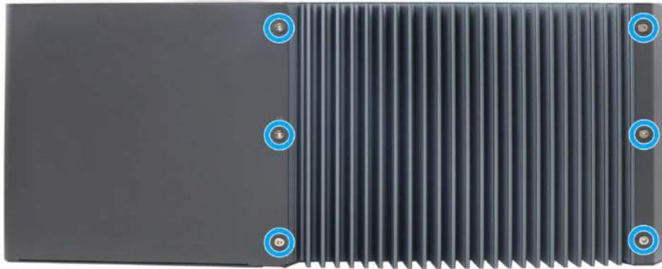
10. Gently lift the heatsink and motherboard upwards to separate it from the enclosure.
