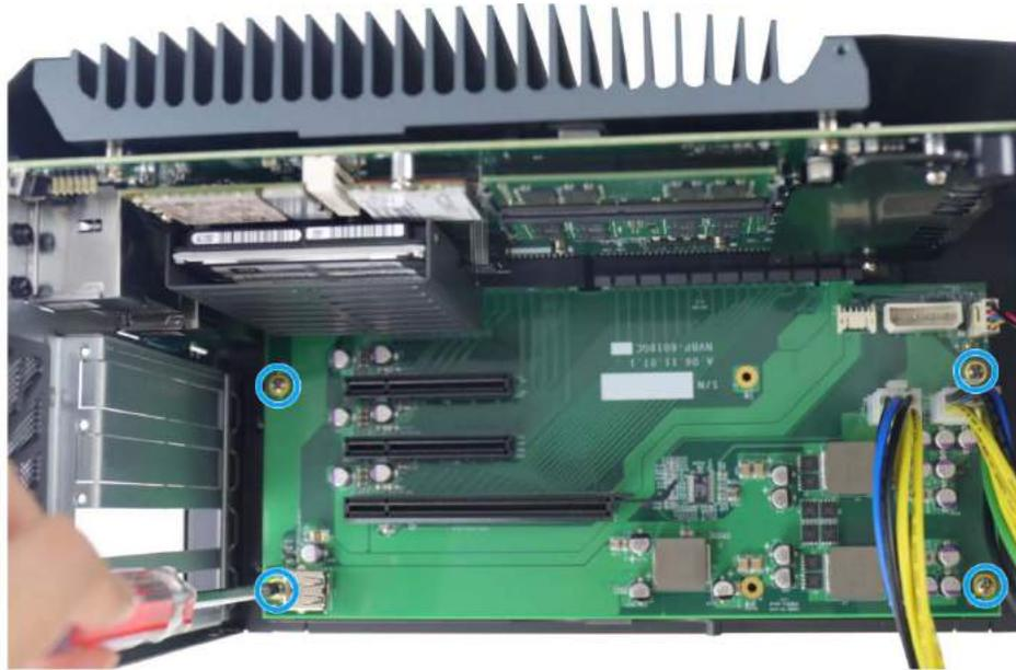
8. Gently disengage the daughter board from the motherboard and out of the enclosure.
