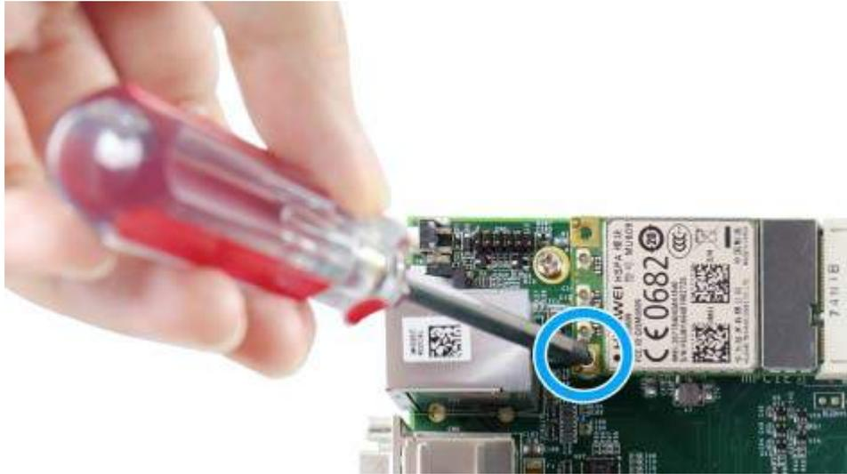
4. Clip on the IPEZ-to-SMA cable to the module and secure the antenna to the rear panel. Please refer to the module's manual for clip-on connection.
