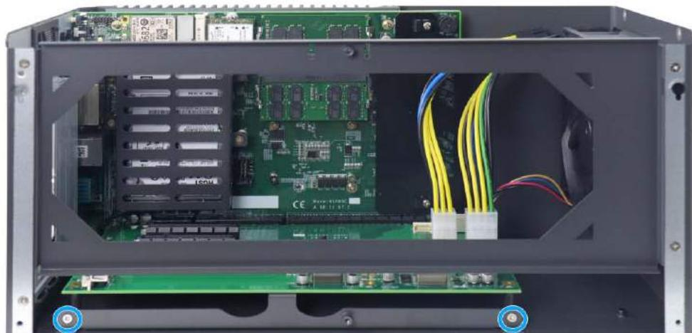
3. Align the HDD/ SSD to the preset screw holes (4 per drive) and secure the drives onto the tray using flathead screws.
