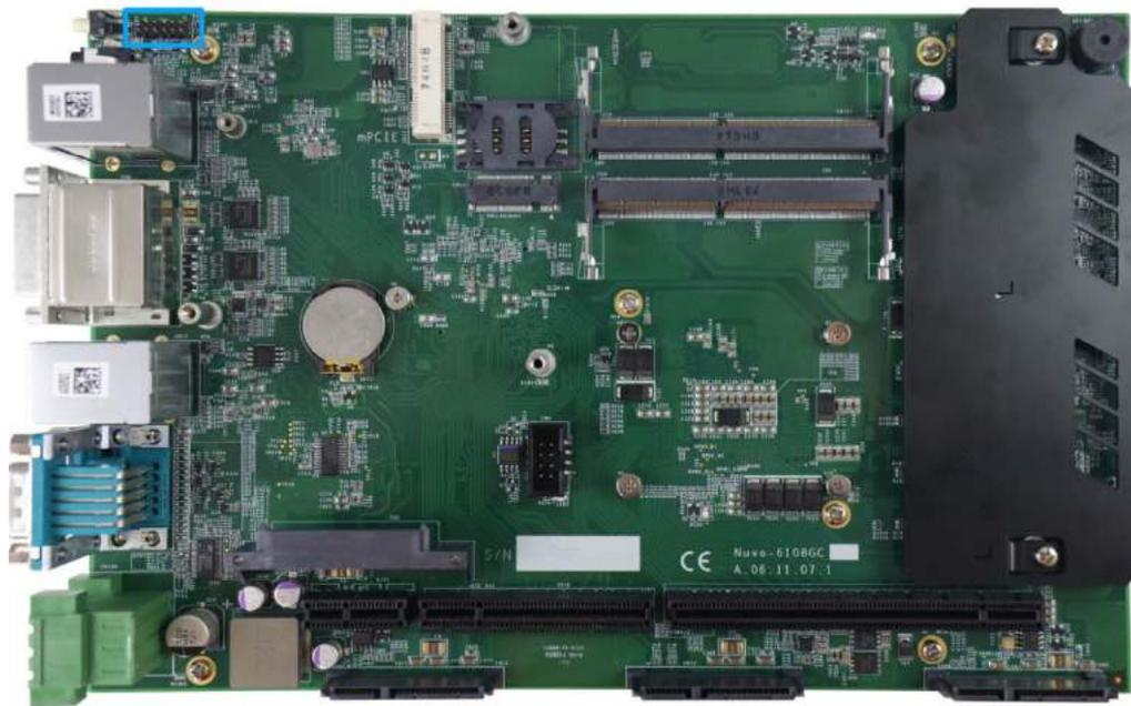
For an application which places the system inside a cabinet, it's useful to have an external system status LED indicators. The system provides a 2x6, 2.0mm pitch pin header to output system status such as power, HDD, watchdog timer, and control system on/ off remotely.
