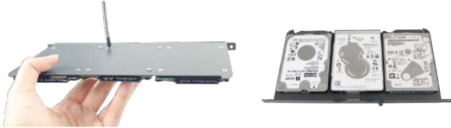
**Use flathead screws to secure drive(s) Drive(s) secured on the tray**
