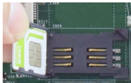
Insert Mini-SIM card with pins facing up
