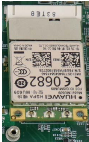
Insert on 45 degree angle
