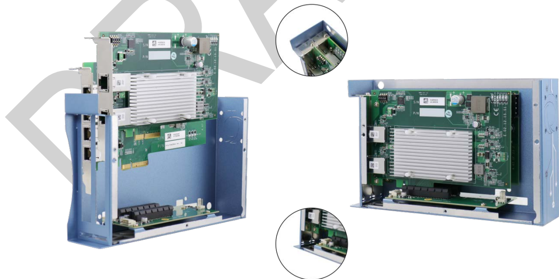
Nuvo-7000DE systems have two PCIe slots in the Cassette module
