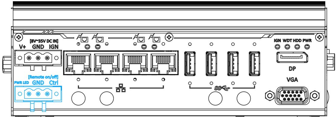
The “Remote On/ Off” 3-pin connection allows for external switch extension. It is useful when the system is placed in a cabinet or a not easily accessed location. You may connect an external remote with an external status LED indicator (15mA) by connecting to PWR LED and GND.
