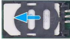
**Close and push towards the outside of the MezIO™ module to secure the SIM card**
