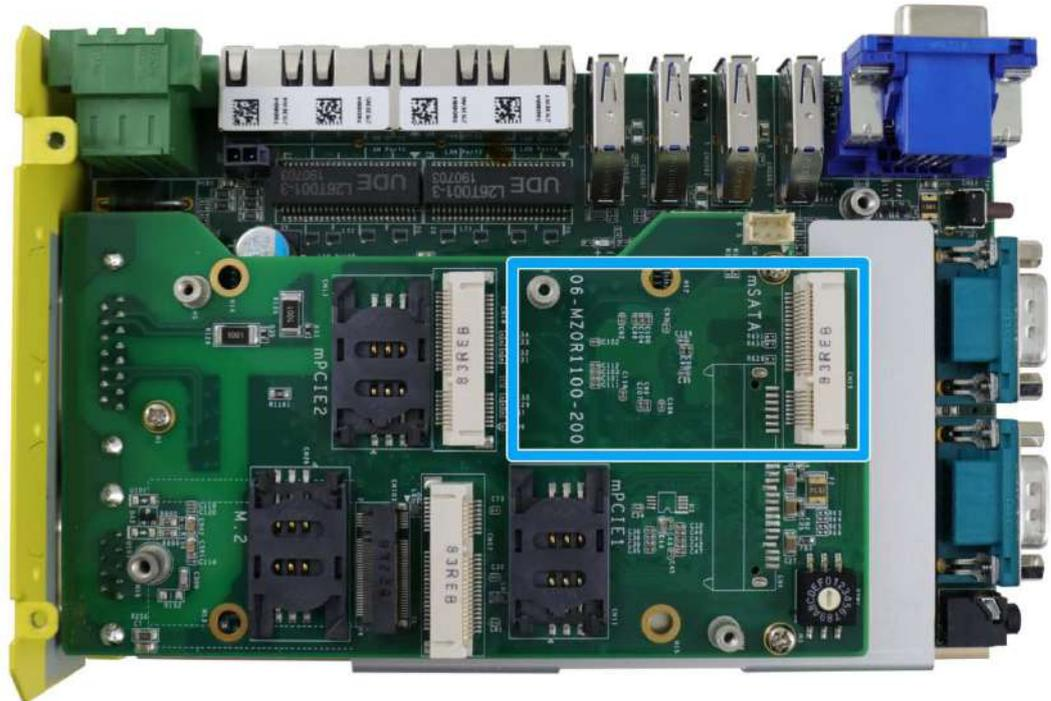
3. Insert the mSATA card on a 45 degree angle and gently press the card down and secure with a screw.
