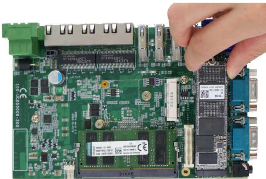
4. Gently push it towards the motherboard and secure the NVMe SSD with the supplied screw.
