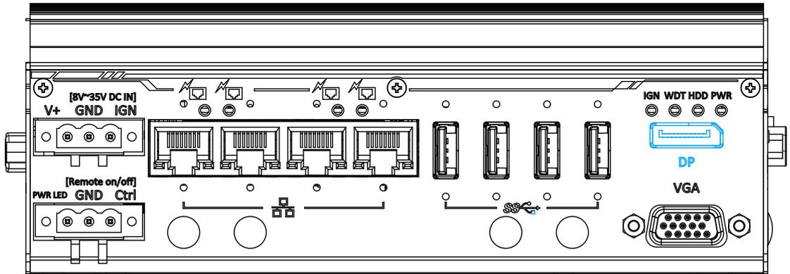
The system has a DisplayPort (DP) output which is a digital display interface that mainly connect video source and carry audio to a display device. When connecting a DP, it can deliver up to 4K UHD (4096 x 2160 @ 30Hz) in resolution. The system is designed to support passive DP adapter/ cable. You can connect to other display devices using DP-to-HDMI cable or DP-to-DVI cable.
