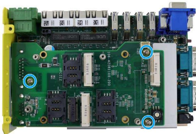
4. As the SIM card is situated underneath the mini-PCIe module, please install the SIM card first. The SIM card slot utilizes a slide-and-clamp mechanism. Slide the top section away from the VGA port, flip open the slot and insert the SIM card.
