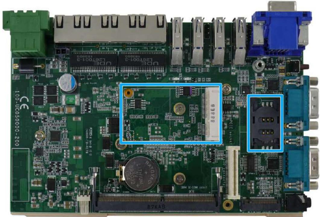
The system provides a full-size mini-PCIe socket. The mini-PCIe socket is designed with SIM card support. With a SIM card installed, your system can access the internet via your network provider's 3G/ 4G network.
