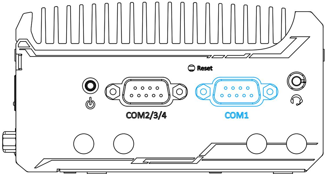
Implemented using industrial-grade ITE8786 Super IO chip (-40 to 85°C) and provide up to 921600 bps baud rate, COM1 is a software-configurable RS-232/422/485 port via 9-pin D-Sub male connector. The operation mode, slew rate and termination of COM1 can be set in BIOS setup utility. The following table describes the pin definition of COM ports.
