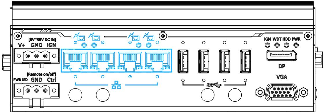
The Gigabit Power over Ethernet (PoE) port supply power and data on a standard CAT-5/ CAT-6 Ethernet cable. Acting as a PSE (Power Sourcing Equipment), compliant with IEEE 802.3at, each port delivers up to 25W to a Powered Device (PD). PoE automatically detects and determine if the connected device is PoE PD or not before supplying power, making it compatible with standard Ethernet devices as well.
