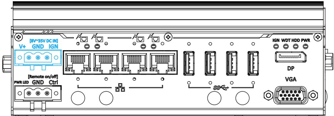
To have ignition power control for in-vehicle usage, you need to supply IGN signal to the system. The IGN input is located on the 3-pin pluggable terminal block (shared with DC power input). For in-vehicle ignition control wiring, please do the following:
