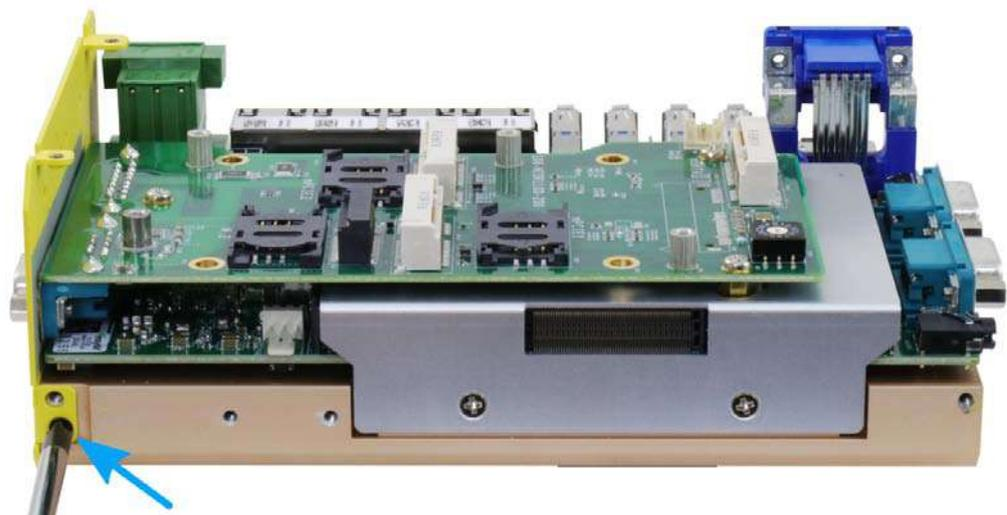
6. Remove the three screws securing the MezIO™ module and gently lift the module to separate it from the mainboard.
