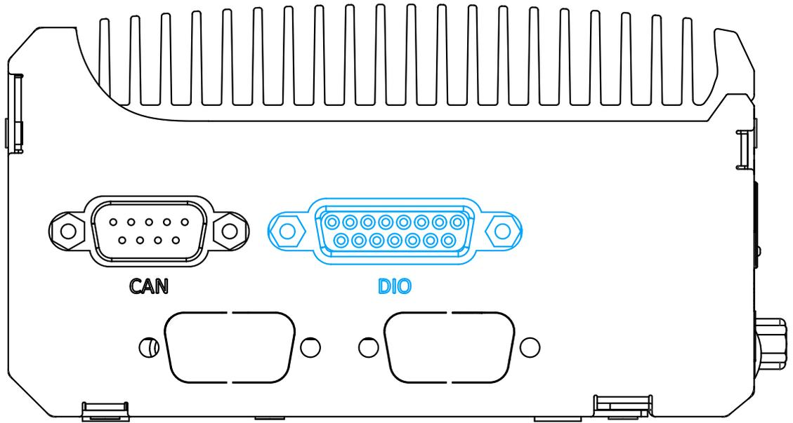
The system provides 4x isolated digital input channels and 4x isolated digital output channels. The DIO functions support polling mode I/O access and DI change-of-state interrupt. Please refer to [Watchdog Timer & Isolated DIO](#) for information on wiring and programming the isolated DIO channels.
