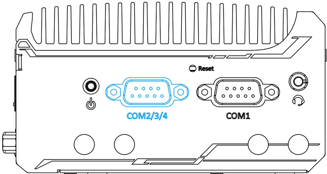
Implemented using industrial-grade ITE8786 Super IO chip (-40 to 85°C) and provide up to 921600 bps baud rate, the D-Sub male connector (COM2/ 3/ 4) can be configured in the BIOS as single RS-422/ 485 port (COM2) or three 3-wire RS-232 ports (COM2/COM3/COM4). Please refer to [COM2/ 3/ 4 Port Configuration](#) for configuring operation mode. An optional 1-to-3 Y-cable is available to connect three RS-232 devices.
