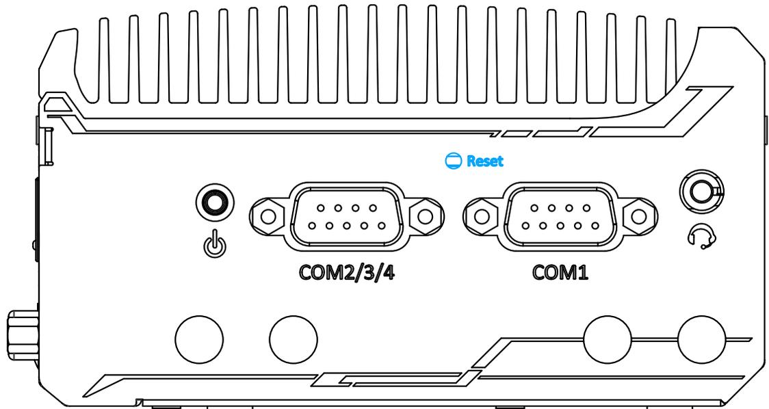
The reset button is used to manually reset the system in case of system halt or malfunction. To avoid unexpected reset, the button is purposely placed behind the panel. To reset, please use a pin-like object (eg. tip of a pen) to access the reset button.
