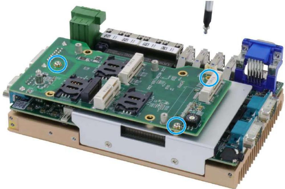
7. Remove the two screws shown below and remove the heatsink covering the DRAM module and M.2 slot.
