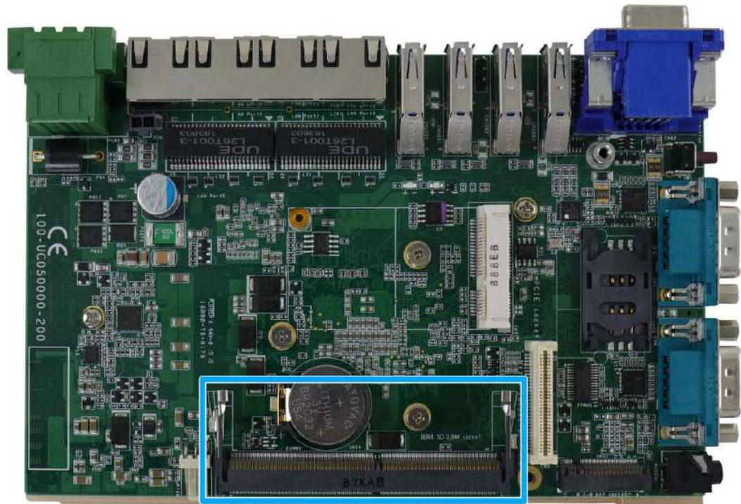
The system supports one 260-pin SO-DIMM socket for installing DDR4-2400MHz memory module up to 16GB in capacity.
