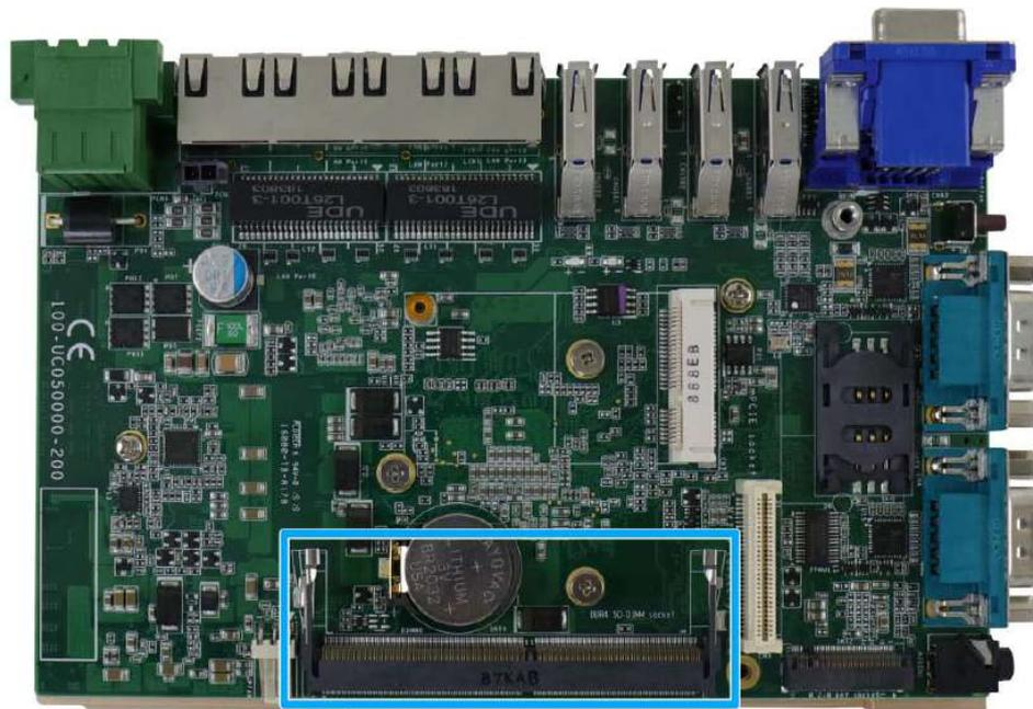
3. **To install**, insert the gold finger end of the SO-DIMM on a 45 degree angle into the slot and gently push the SO-DIMM down until it is clipped-in.
