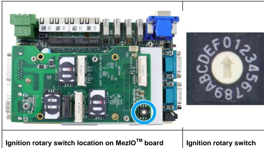
[The ignition control module is also BIOS-configurable.](#) When rotary switch is set to mode 15 (0xF), the ignition power control is set to executed according to parameters configured in BIOS setup menu, which allows richer combination of power-on/power-off delay and more detailed control parameters.
