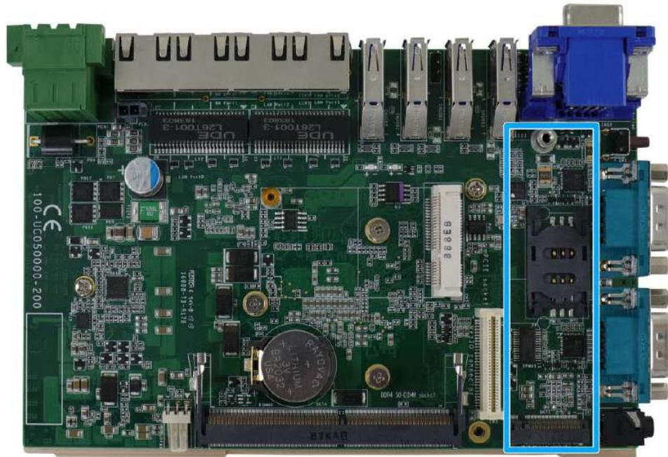
3. Insert the NVMe SSD into the slot on a 45° angle.
