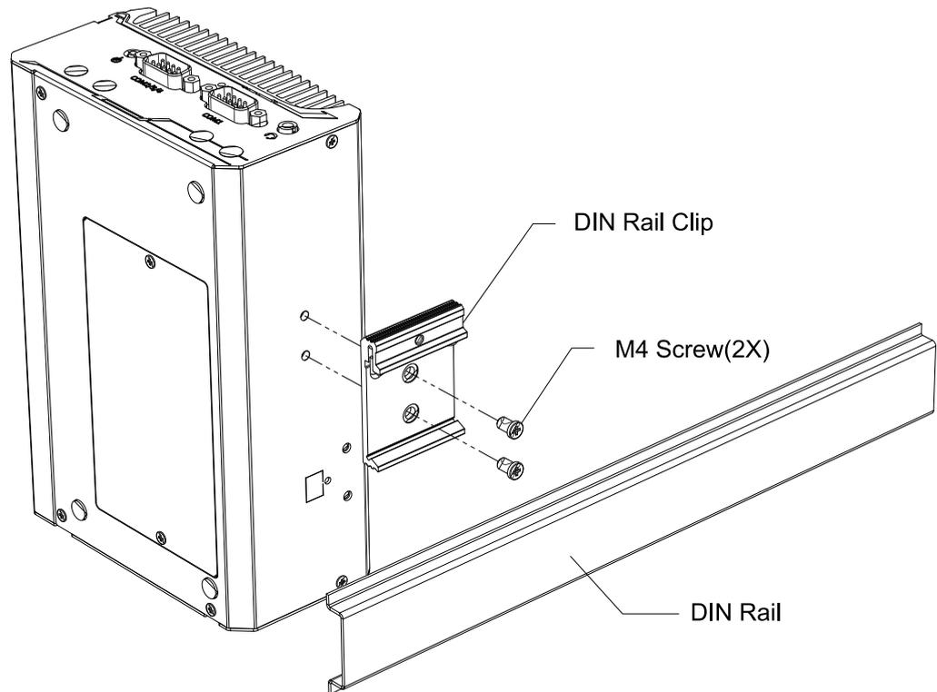
2. To install the DIN rail clip onto the DIN rail, you must come over the top of the DIN rail, tilting, overlap the top clip edge of the DIN rail clip onto the DIN rail first, and then firmly press the bottom-front of the enclosure to clip the bottom edge of the mount plate.
