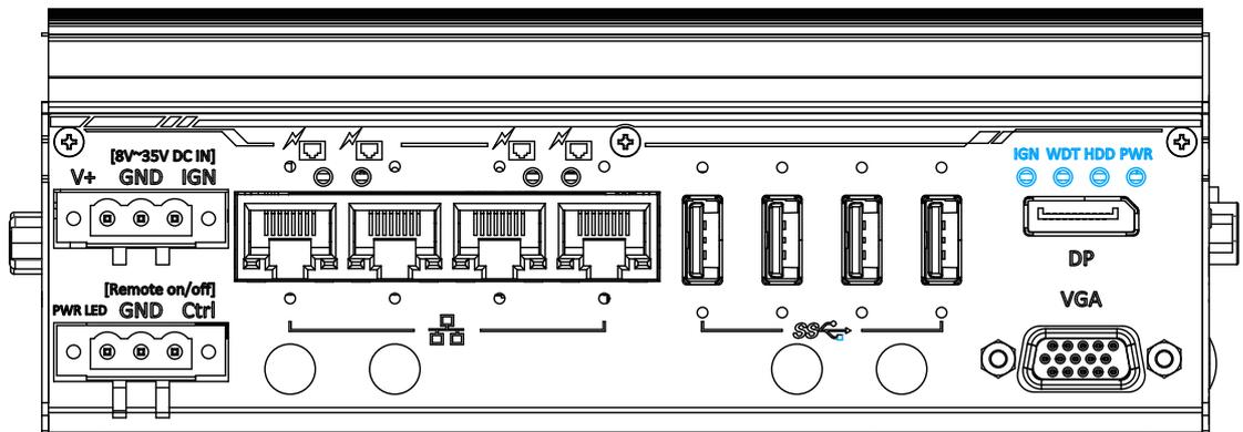
There are four LED indicators on the front panel: IGN, WDT, HDD and PWR. The descriptions of these four LEDs are listed in the following table.
