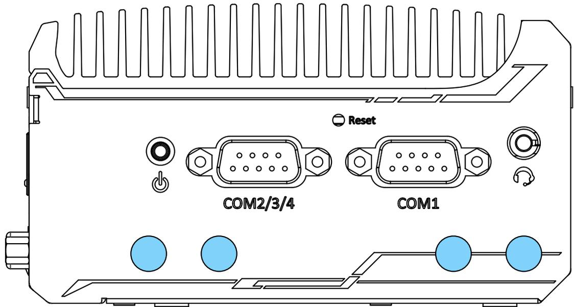
The system offers four SMA antenna openings reserved for SMA antenna installations. Users can take advantage of these three openings when installing mini-PCIe module for wireless communication reception such as 3G, 4G, GPS or WiFi.
