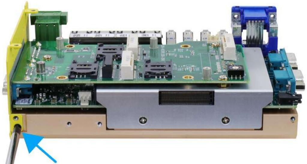
2. Install the front panel by securing it with three screws and two hex-bolt screws on the VGA connector.
