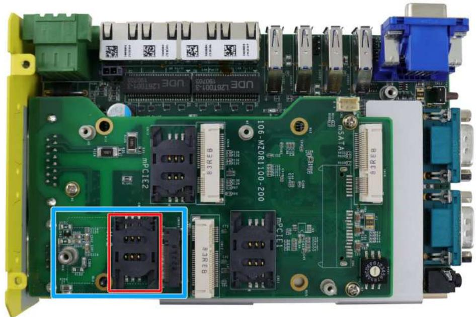
3. To insert a SIM card, push and flip the slide-and-clamp slot towards the center of the MezIO™ module.
