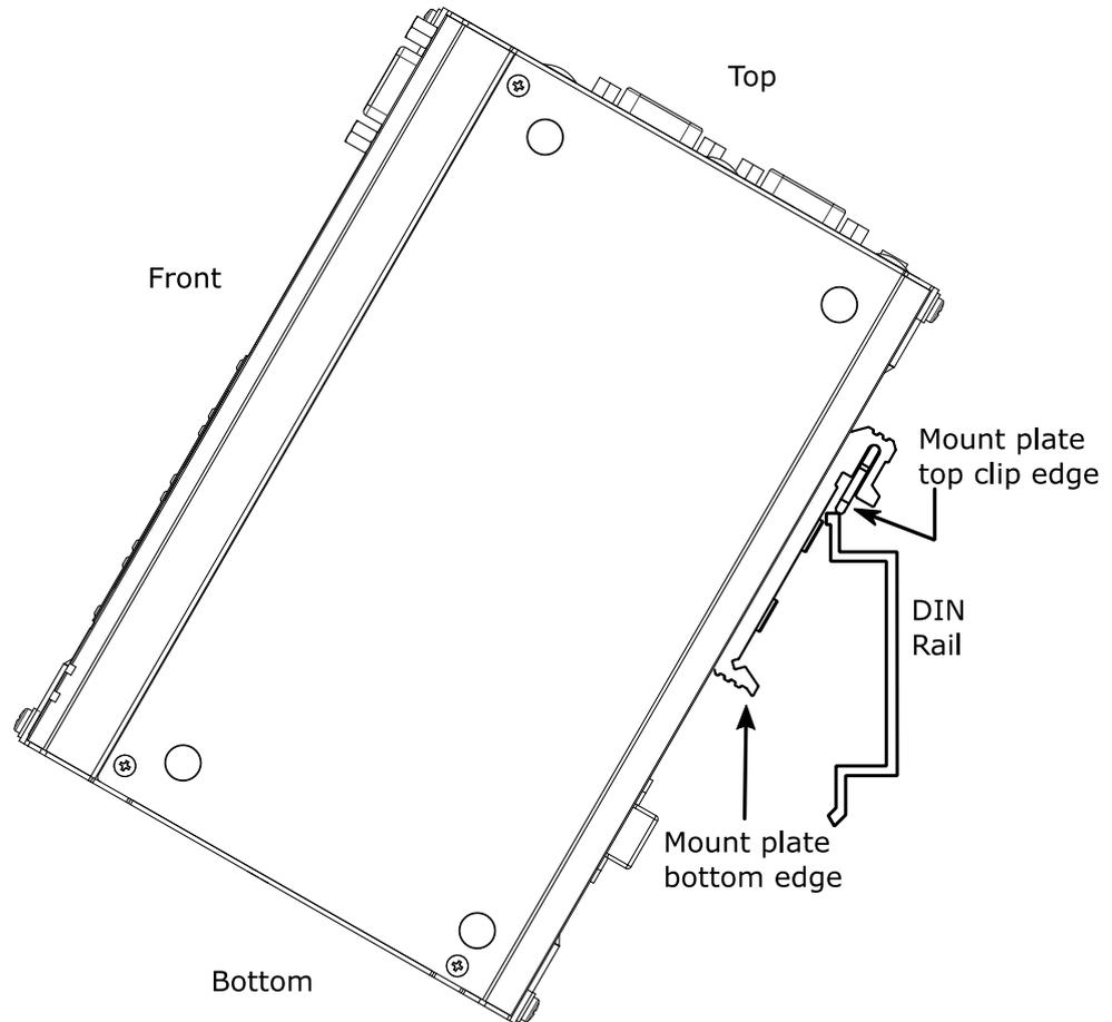
3. Confirm the mount plate has indeed clipped onto the DIN rail for proper fit to complete the installation.
