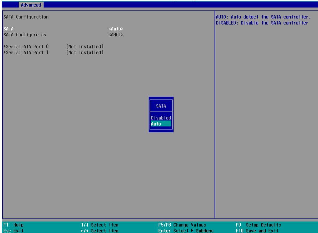
The SATA configuration setting should be configured according to the MezIO™ card installed. For detail settings, please refer to the following table.
