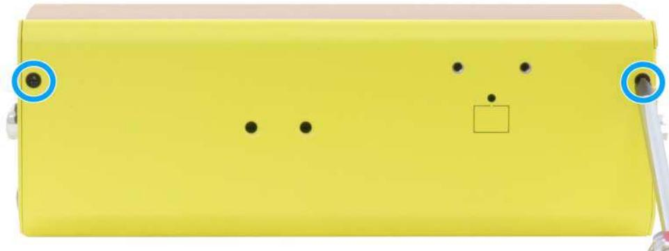
4. Turn the system upside-down, remove the three screws indicated and separate the L-shape enclosure panel from the heatsink/ mainboard.
