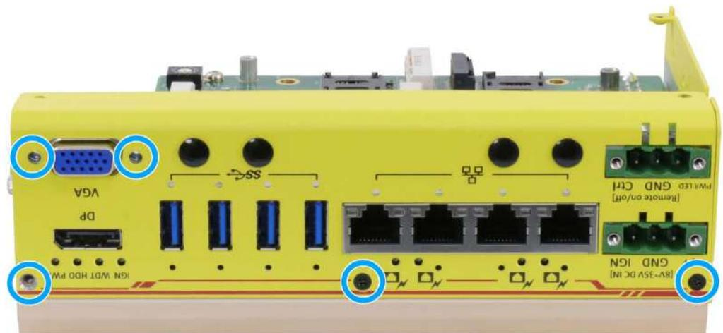
3. Place the L-shaped enclosure panel back into place and secure it with three screws.
