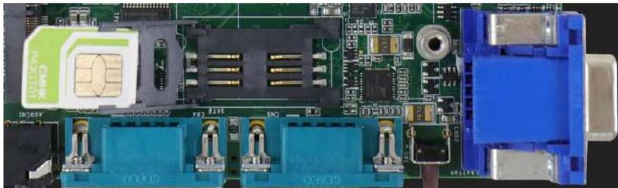
**Flip open the slot and inset SIM card**
