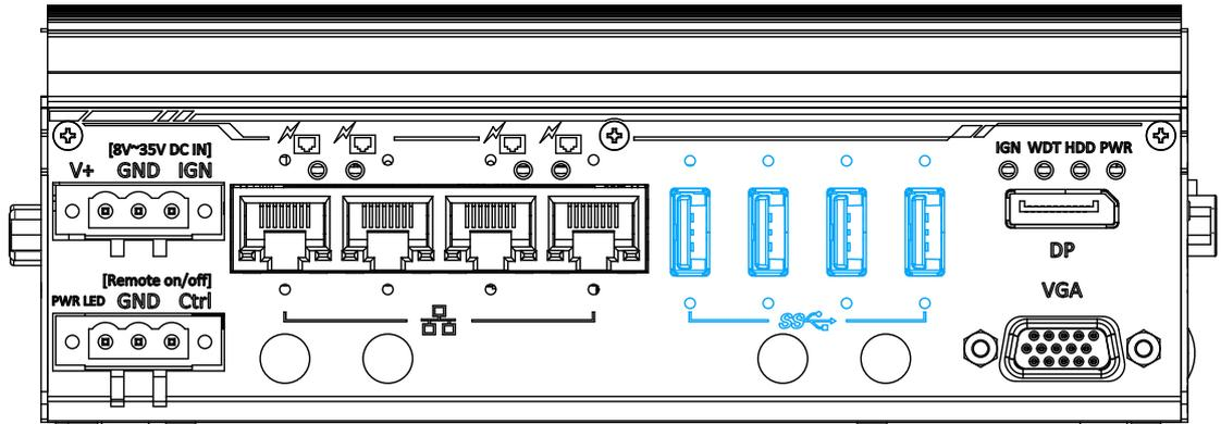
The system offers four USB 3.1 Gen1 (SuperSpeed USB) ports on its front panel. They are backward compatible with USB 2.0, USB 1.1 and USB 1.0 devices. Legacy USB support is also provided so you can use USB keyboard/mouse in DOS environment while USB 3.1 Gen1 driver is supported natively in Windows 10.
