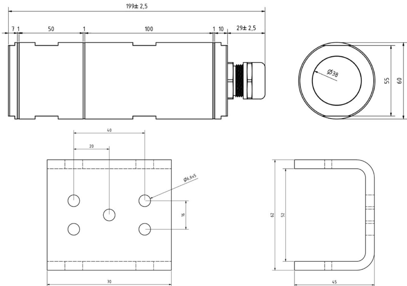
Standard dimensions of the housing and mounting bracket (mm).
